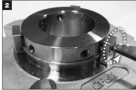
Remove the centering clips and discard.
