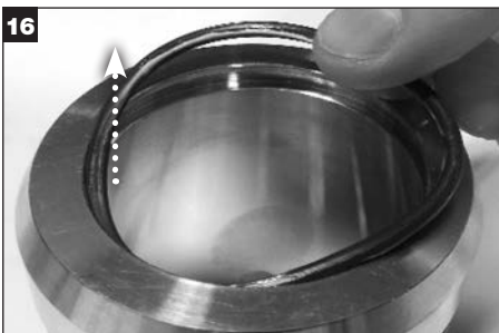
Remove the shaft O-Ring (V) from the sleeve and discard.
